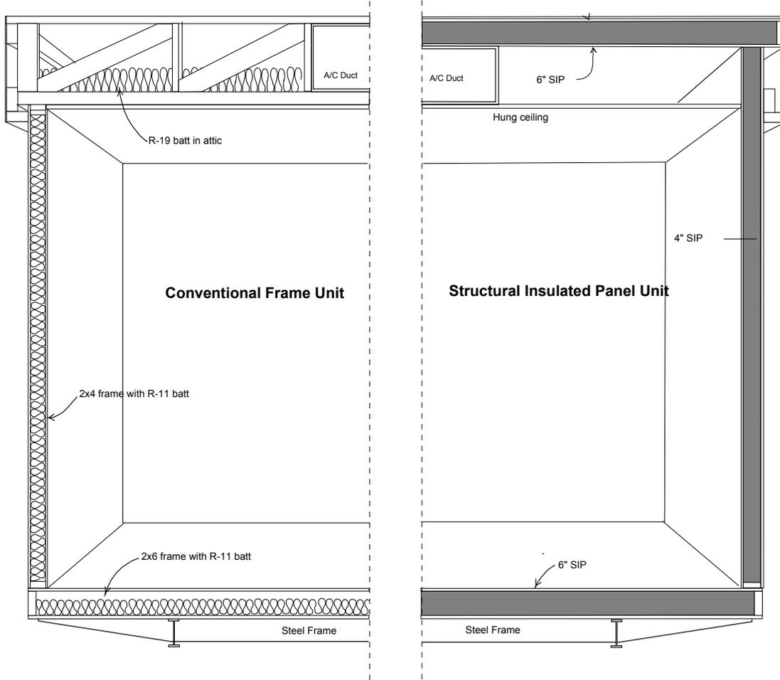
Schematic cross-section through the modular offices, frame unit on the left, SIP unit on the right
