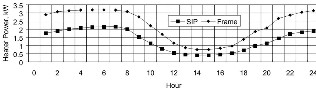
It is informative to compare the fractional reduction in BLC, peak demand, and energy use between the frame and SIP modules. In general these values should be similar, but not exactly the same because of solar energy and heat storage effects.
