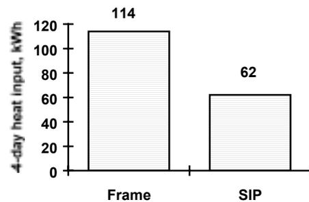
The weather was sunny during these 4 days. The average outside temperature was 48°F, and the average temperature inside both units was 73°F. The total electricity used (which includes a small amount of electricity for the data logger and the fans) was 114 kWh for the frame unit and 62 kWh for the SIP unit (Figure 15). The SIP unit used 46% less energy than the frame unit.
