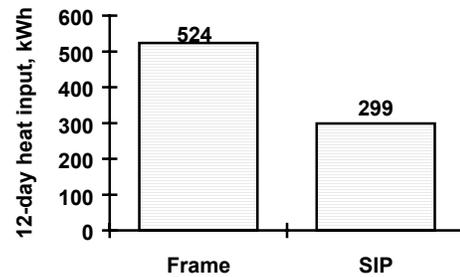
This period included one cold night following a cloudy day. The minimum outside temperature at 5 AM was 16°F, and the inside temperature was held at 70°F. The peak power at this time was 5.26 kW in the frame unit and 3.28 kW in the SIP unit. The peak for the SIP unit was 38% lower than for the frame unit.
